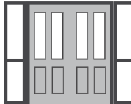
Double Doors with Glazed Sidelights and Midrails
