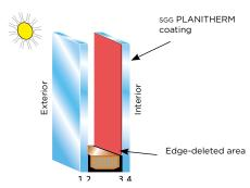
Insulating glass unit with sGG PLANITHERM (coating on face 3)
