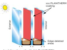
Insulating glass unit with sGG PLANITHERM (coating on faces 3 and 5)
